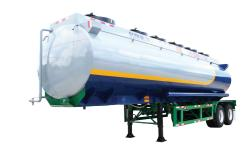
CEMENT TANK SEMI TRAILER, 30.12 M3, 40 FEET, 03 AXLES
